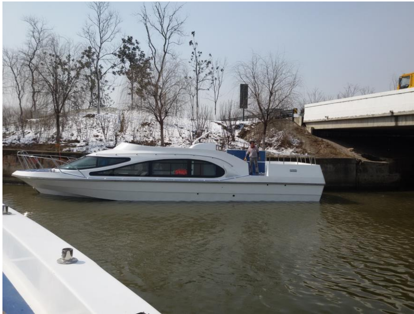
HD-1380-Price:117000USD Includes Global Shipping Over length: 13.8m Beam: 3.5m Depth: 1.2m Dry weight: 5600kg Seats:33+2 Engine: Cummins Diesel Inboard 260hp (shaft with propeller)
